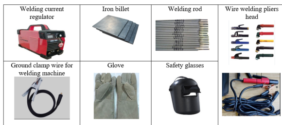
Figure 4. Some tools and equipment commonly used in flat position butt welding.
