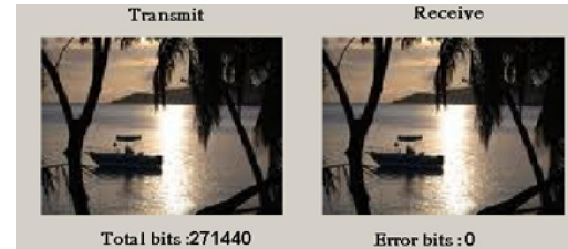
Figure 8. Simulation without channel estimation, SNR=20 dB, 4-QAM with only Gaussian noise impact
