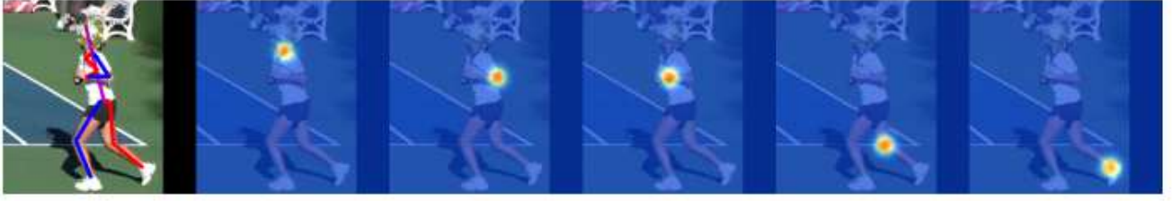
Figure 2. Illustration of heatmaps predicted from human body image. Therein, each heatmap is a candidate prediction of keypoint locations (x, y) [28].
