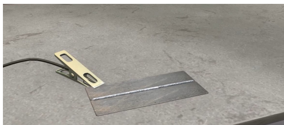
Figure 10. Image of the butt-welded metal plate in the flat position after the slag has been removed.
