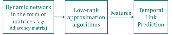
Figure 31. Principle of temporal matrix factorization model
